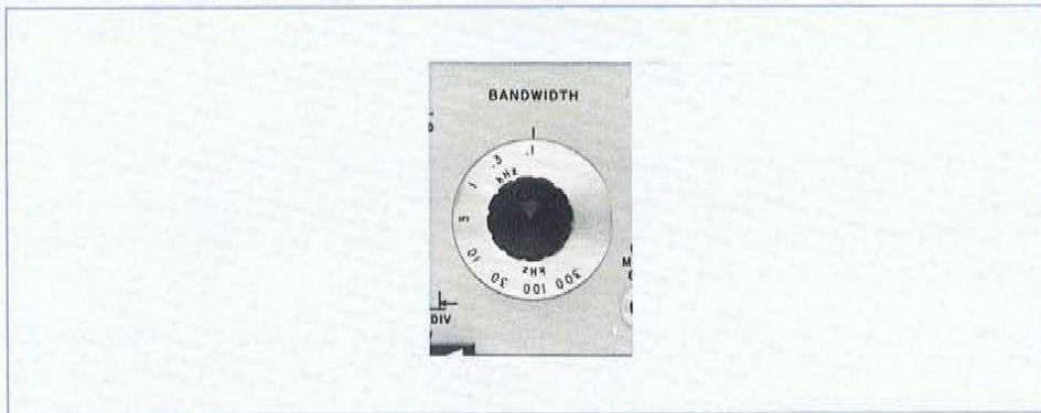
Figure 9. The setting of the bandwidth control is the nominal 3 dB bandwidth of the spectrum analyzer.
